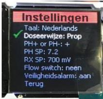
Press the bottom key. The "dosing mode" setting is now checked. Press the middle key to activate this setting. You can now see that the dosing prop (= proportional) is selected. Press the middle key again. The dosing proportionally is now set.
