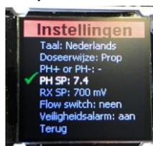
Press the bottom key. The "PH SP" setting is now activated . Press the middle key to activate this setting. You will now see a preset value. Now you can use the upper or lower key to set the value higher or lower, after which you can confirm by pressing the middle key. The value is now set to your wanted value
