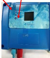
As soon as the calibration starts, a screen lights up, showing you what you are calibrating. You can either only calibrate Ph or calibrate only Rx or calibrate both at the same time.
