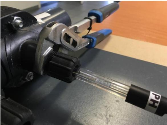
**3**) Connect water inlet and water outlet so that the water first passes the pH measuring probe and RX measuring probe and then passes the Ph and Redox dosing (according to the direction of the yellow arrows on the tube). This is the preferred bypass configuration installation:
