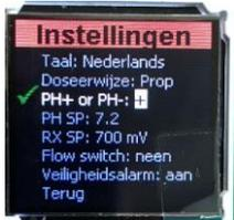
Press the bottom key. The "PH+ or PH-" setting is now active. Press the middle key to activate this setting. A sign - appears. Press the middle key again. You have now set the pH -.
