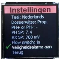
The alarm function is necessary to warn the user of abnormal behavior of the device, and to prevent, for example, a very large dose of pH liquid or too much chlorine being produced.
