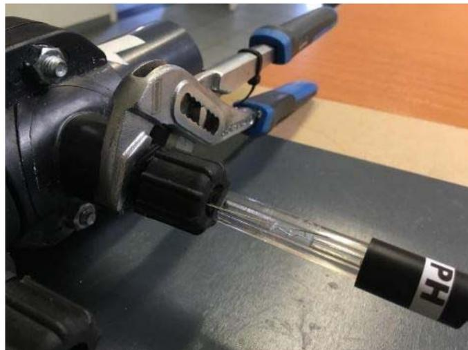
3. Connect water inlet and outlet so the water first passes through the redox and pH measuring electrode and then along the salt electrolysis.
